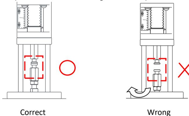
**Solution:** Rotate the Valve Stem Adaptor in the CW direction until the bottom adaptor touches the surface of Actuator Stem Adaptor.
