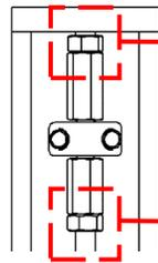
Secure the Actuator Stem Adaptor and rotate the Actuator Nut until tight.
